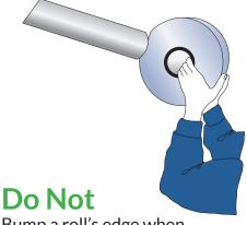
Bump a roll's edge when placing it on a mandrel.
